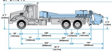
A convenient switch of hoses using the optional SBU rod/piston conversion system allows the user to go from the rod side to the piston side quickly and easily. Capable of pumping pressures up to 3,200 psi (220 bar) on the piston side, the CP 2110 HP can handle a range of applications including high-rise jobs.
